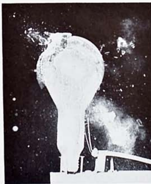
A result of an R. G. & E. employe's high-speed photography is this picture of a light bulb being smashed by a B-B shot. The two electrical contacts can be seen to the right. These contacts start the electronic impulse which causes the emission of a high-intensity light necessary for this type of photography.
