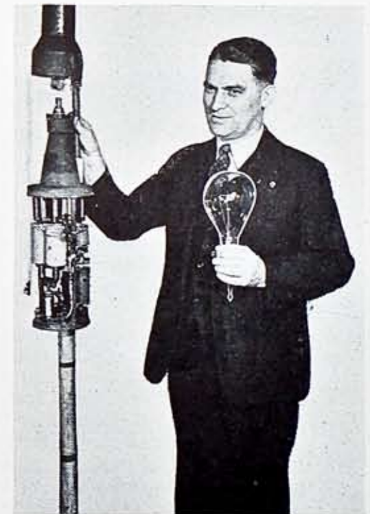
Walter Paine supporting the inside mechanism of one of the now discarded Edison Arc Lamps. The comparatively insignificant looking lamp bulb Walter holds in his left hand does as much lighting as the entire contraption it now renders obsolete.
