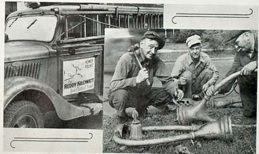
Bill Haggerty, Harry Miller and Howard Walters, of the Underground Department, doing a little "chiseling" in order to make one good harp-type lamp fixture out of three old ones. They took off their goggles so that the photographer could tell them apart, as "REDDY KILOWATT" looks on at the left.
