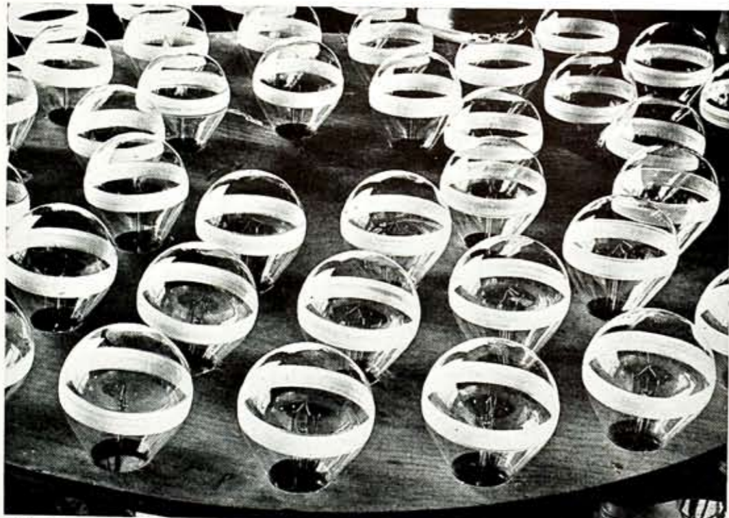
The lamps, after the band is coated about them to prevent glare to pedestrians and drivers from the filament of the plain (non-frosted) lamps are dried by being circulated in the merry-go-round arrangement shown above. An electric fan circulates a draft of air and dries the lamps as the table rotates.
