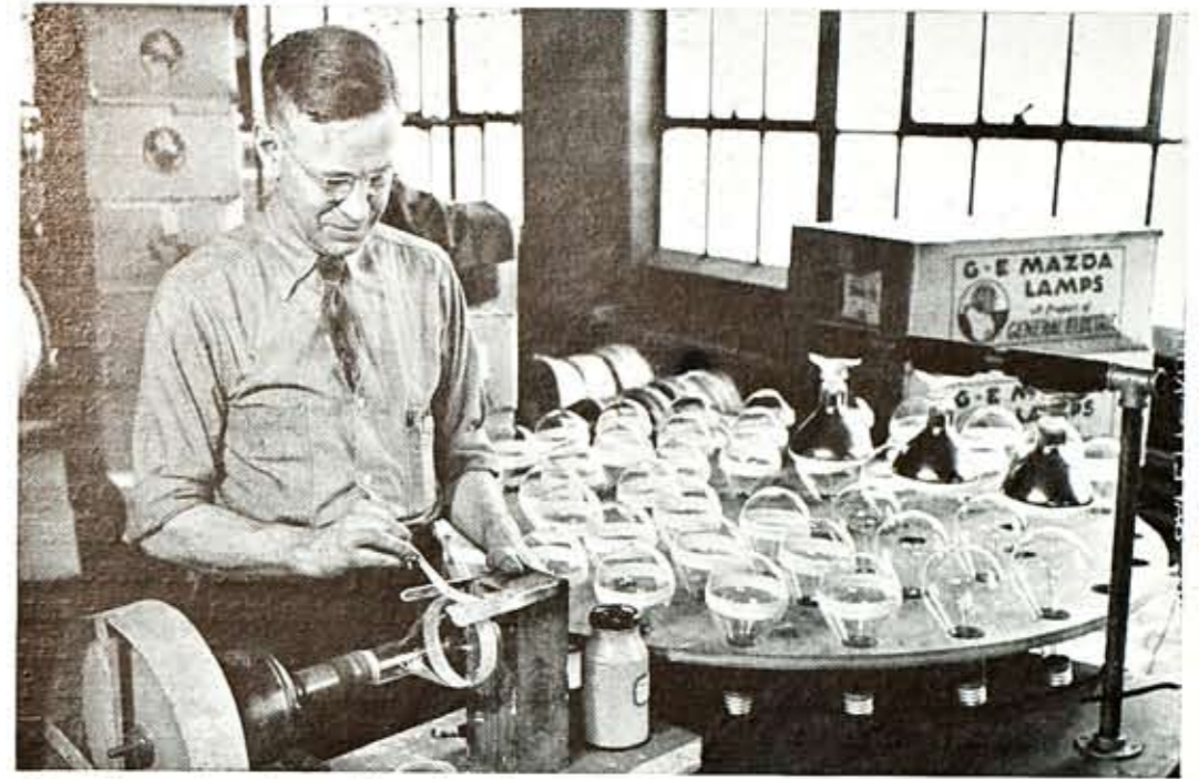
Bert Hammond applies coating paint to lamp rotating in a turning lathe-like machine invented by Company employees. About 40 cases or 960 lamps can be coated per day. This costs less per lamp than was paid for the inside frosted lamps which can not be obtained because of wartime restrictions on materials.
