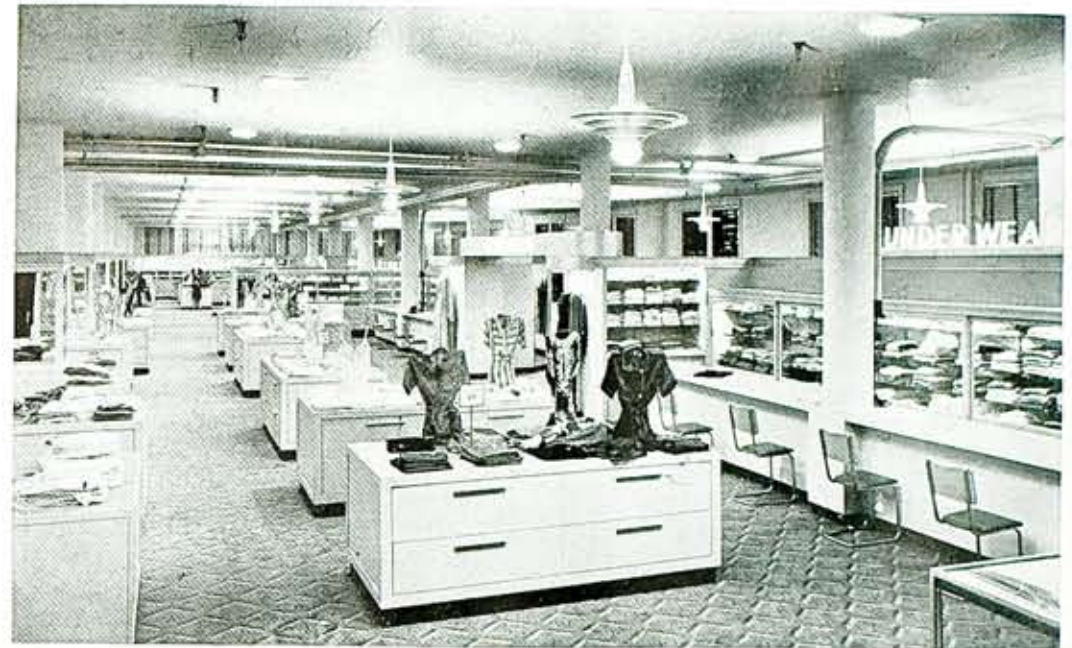
Third floor at McCurdy's. A modern decorative scheme, coupled with lighting from both built-in louvered fixtures and from ceiling suspension luminaires of the direct-indirect type provides comfortable lighting, comparable to that experienced in the shade of a tree on a bright summer day.
