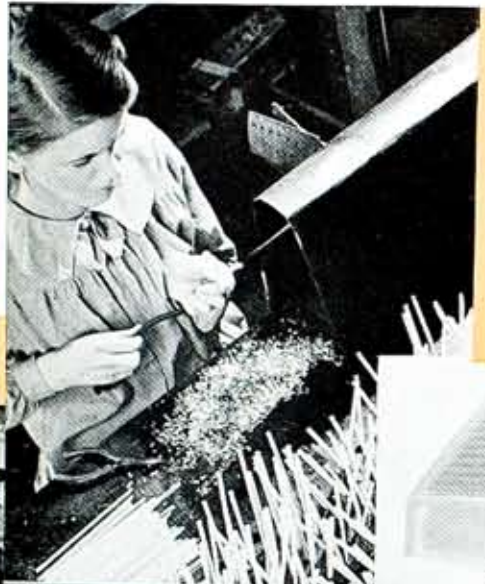
Left, "A drop of mercury, a tube of glass." A step in the making of TAYLOR Thermometers.
