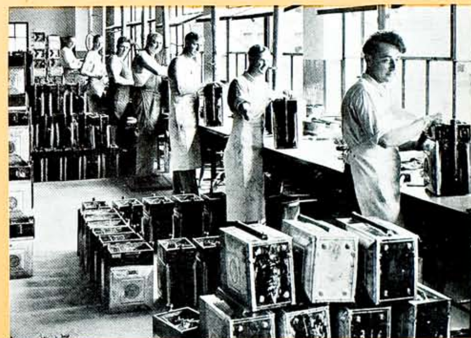
Section of Front Street Gas Shop where gas meters are inspected and repaired at intervals prescribed by state regulation.
