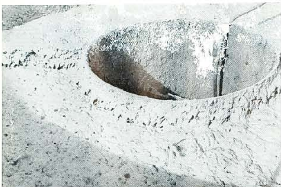
Bubbling mass of solution at East Station Thionizer's top, where sulphur is released into the circular space and run off into a nearby building.
