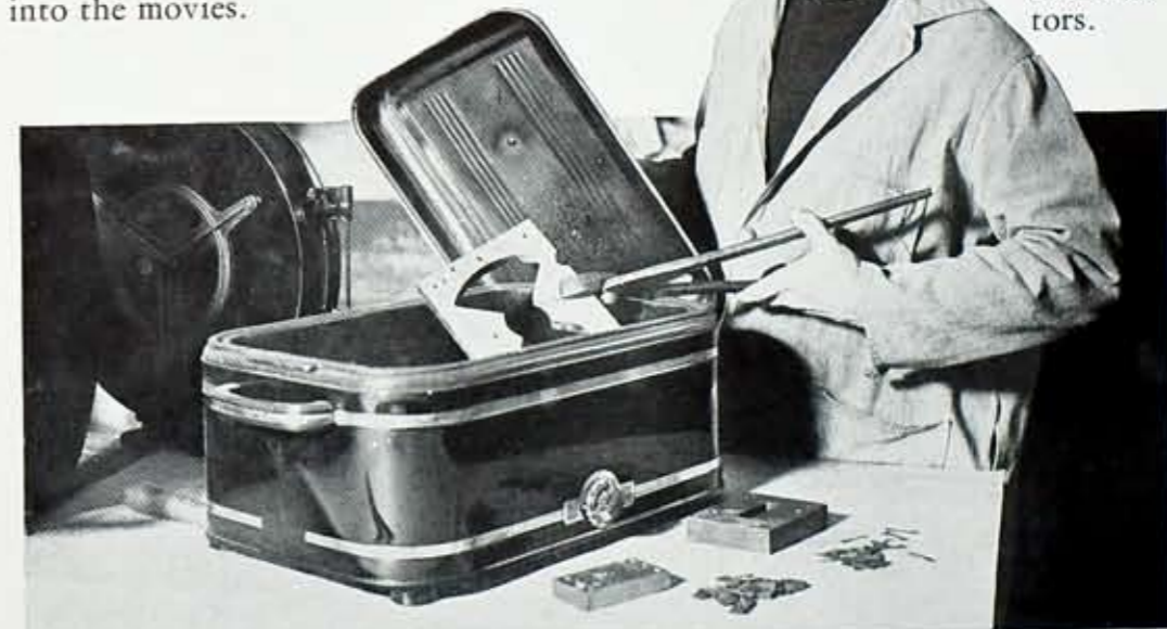
Showing a Westinghouse de luxe Adjust-o-matic electric roaster, (or, "chicken cooker") being used at the Weber Machine Corporation in the tempering of small parts for the "Syncrofilm" sound projector, a job which it does exceedingly well.
