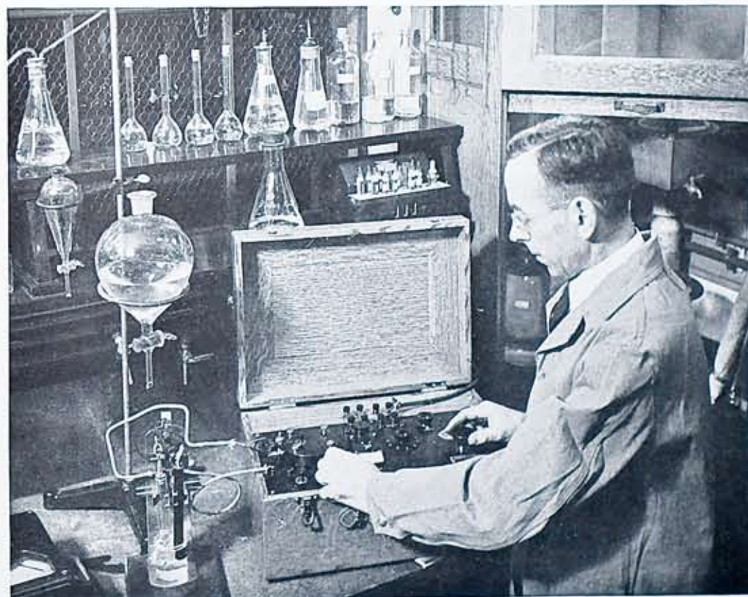
These pictures show typical scenes in the chemical laboratory, top, at East Station and bottom, the chemical laboratory at Station 3 Extension. Messrs Louis Shnidman and Frank Henry, respectively, are seen carrying out feed water tests for Station 3 boiler water. In the picture at the bottom is seen the new electrometer used in measuring hydrogen ion concentration.
