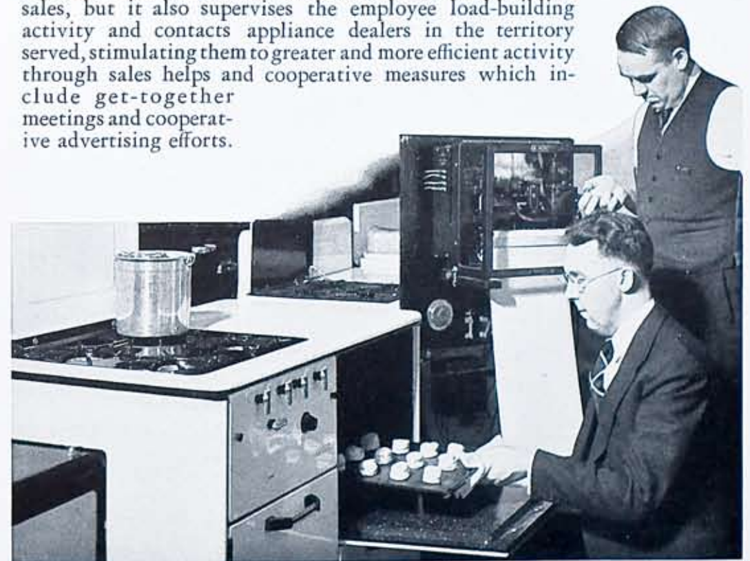
Actual performance tests are given gas ranges in the electrical and gas laboratory, which includes actual baking. Refrigerators are operated for extended periods, and all appliances are accepted or rejected for Company sale on the basis of their actual performance.
