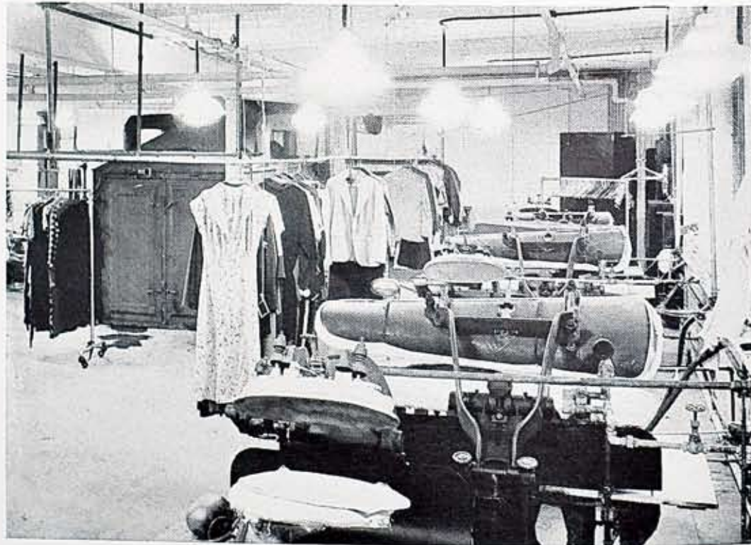
Work must be perfect to pass inspection at Marriotts French Dry Cleaning Works, Inc., 31 River-view Place. There is 25 foot-candles of light on the steam press "shoes" and 45 foot-candles in the left rear corner of the room shown, where hand pressing and spotting is done.
