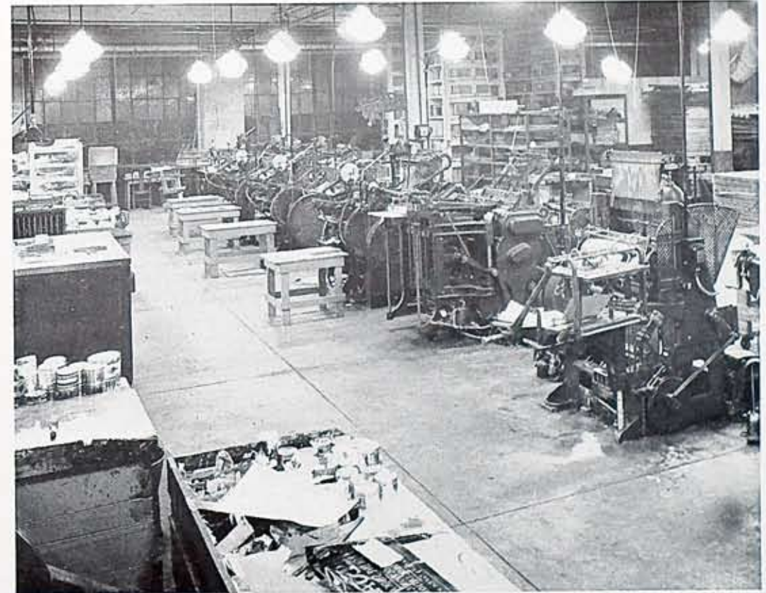
Small section of Bastian Brothers plant, 1600 Clinton Avenue North, all of which is being relighted with 200-watt Glassteel diffusers on eight-foot centers, producing 18 foot-candles of light at the working plane. This is supplemented by local lighting on the machines.
