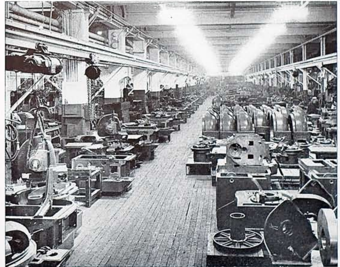
Bottom, Assembly floor at the Gleason Works, 1000 University Avenue, lighted to a level of 15 foot-candles. This is produced by Cooper-Hewitt fixtures, combining a 275-watt mercury tube with four 100-watt Mazda lamps. The resulting light color approaches that of daylight.
