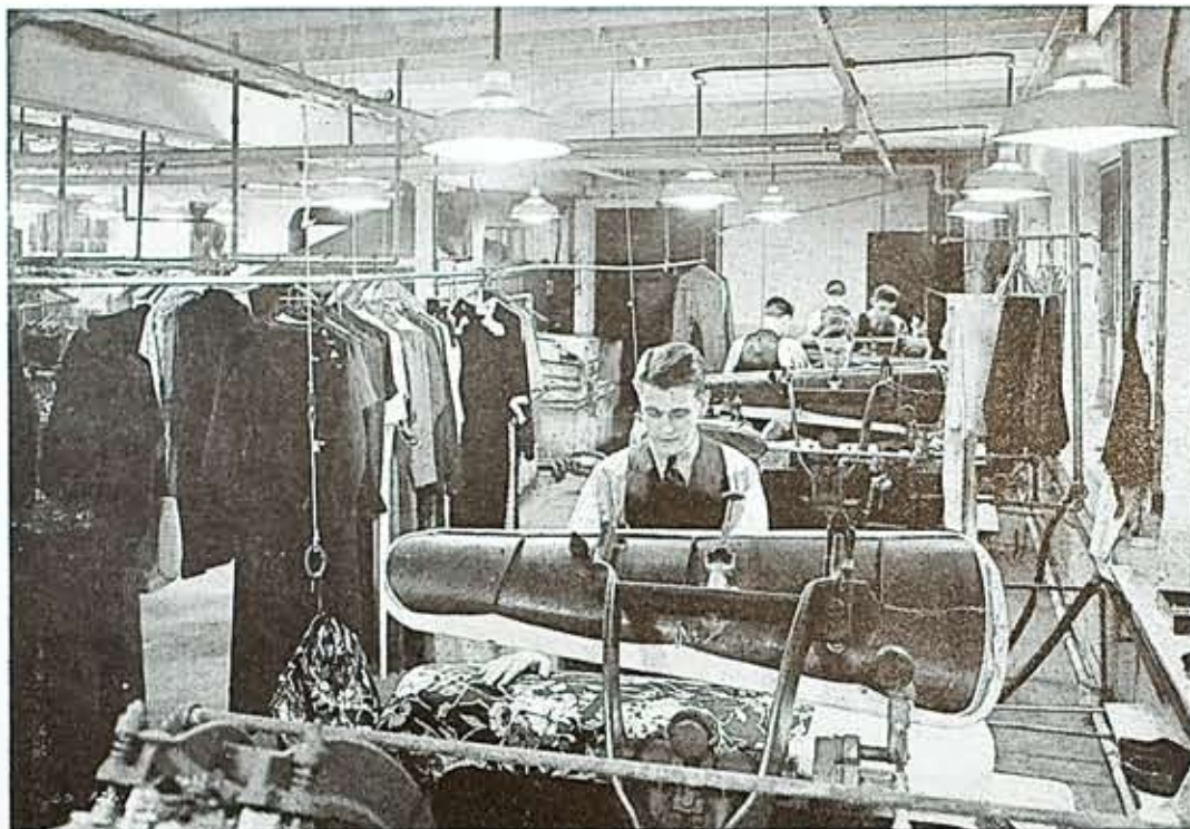
Marriott's cleaning establishment can vouch for the utility of good lighting in finding and eliminating spots on clothing sent in to be cleaned. Good lighting cuts down the number of garments returned by at least one-tenth, while speeding production approximately eight per cent.
