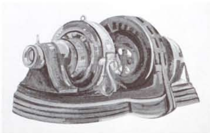
A 500-kw, 2-phase, 2200-volt, 60-cycle motor generator for transforming A.C. to the 3-wire D.C. system. This set was included in the purchase of the Municipal Gas and Electric Company in 1902. Until recently it was in use at Station Four.
