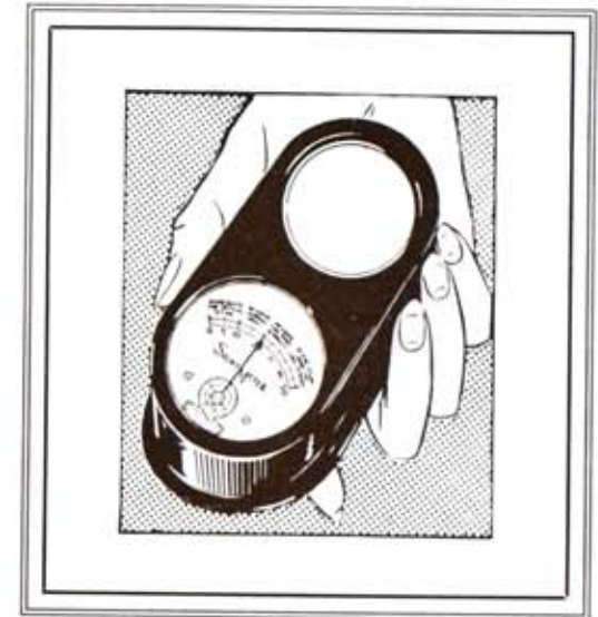
This little device shows whether your lighting is good or if it is causing you to strain or abuse your eyes. It is being used by the Company to help you make sure your lighting is of an intensity required for doing a proper job of "seeing."
