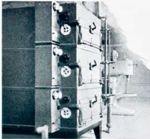
The 18-Kw Westinghouse electric oven.
