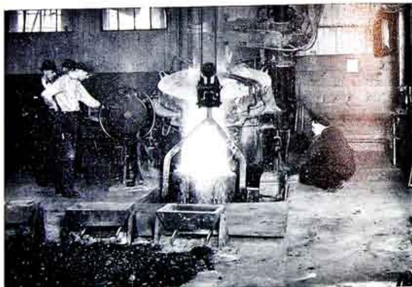
Electric furnace in operation at the plant of the General Railway Signal Company which brought a new industry to Rochester for the production of electric steel castings and low carbon steel castings.
