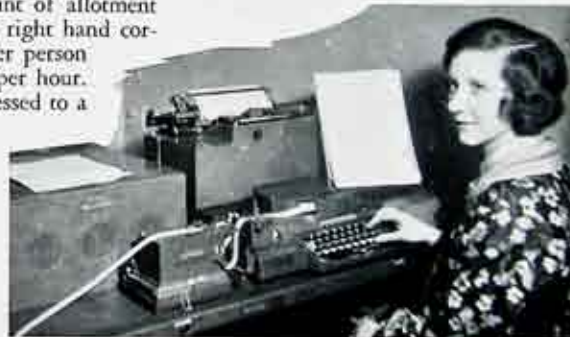
Telephone typewriter device, maintaining, initiating written communication between Ithaca and financial office in New York.
