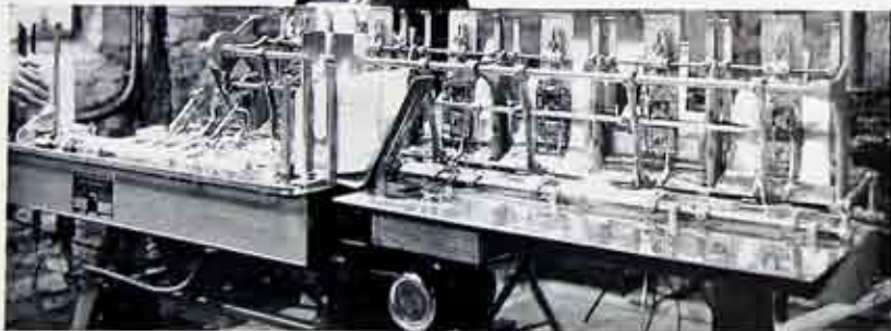
"Latest thing on the market." Inserting machine being installed and which will assemble in high in the enclosure, place in envelopes and seal the flap.
