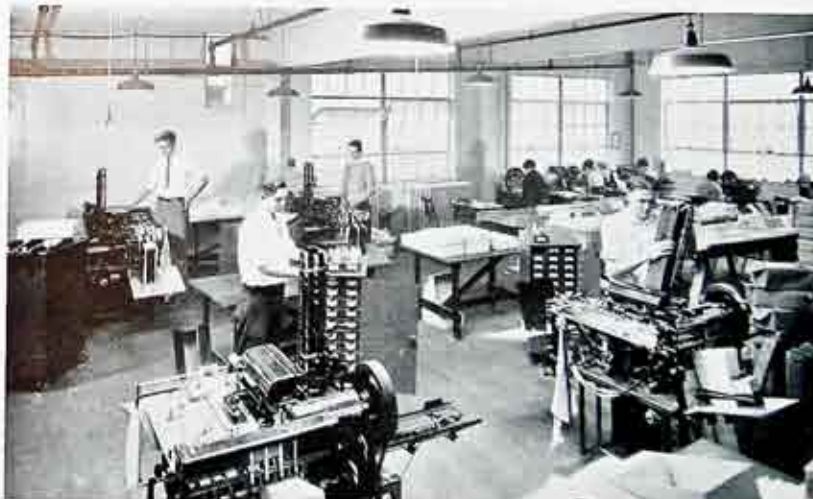
Machine room of Addressograph Division, showing graphotypes (stencil-cutting machines) and automatic addressing equipment.
