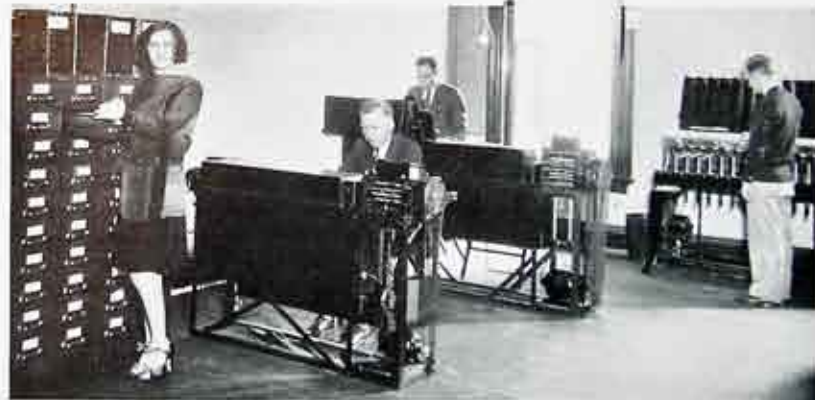
Hollerith tabulating machines, which make possible the payment of dividends to 101,000 Class A stockholders in a period of three weeks.
