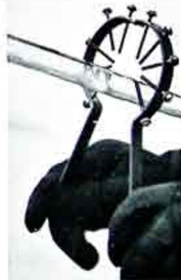
An especially useful instrument in gathering data concerning ice formation on wires, the contour gauge.
