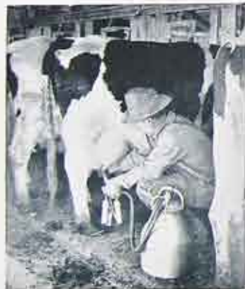
The electric milking machine replaces a hired man for every fifty cows. Not only are cows milked, but they are also groomed and clipped by electrical devices, all of which makes for shorter hours of work, a much cleaner milk supply, and contented cows.
