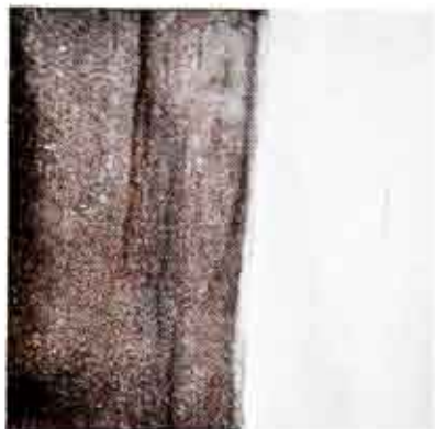
Section of (left) filter paper after one month's operation as compared with (right) a section of the clean filter paper. This dust and dirt is present in most homes, in the air, but filtering extracts it and in the process the home becomes better ventilated.
