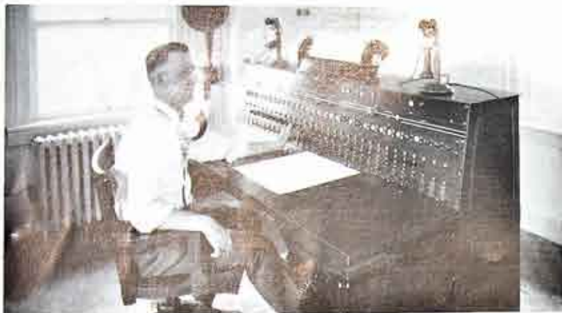
One man, operating this G-R-S Dispatching Machine can follow the progress of trains throughout 40 miles of road, control them and cause them, through the application of electricity to mechanical equipment, to obey his will in the interest of safety, service and dispatch.
