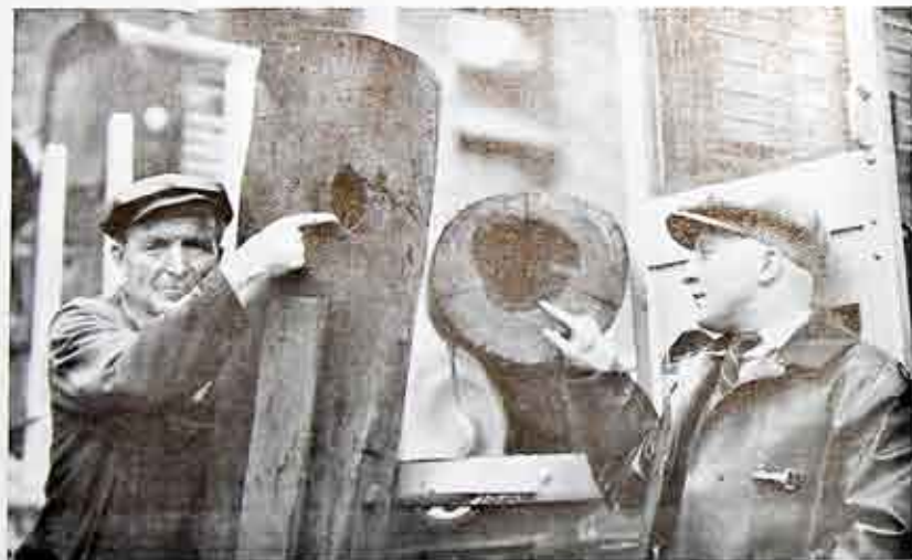
The boom was sawed in two just above the "family" entrance, to which Mr. Charles Ayen is pointing. Mr. John Baker, right, is indicating the woodpecker's "pantry," or the danger zone in the decaying boom.
