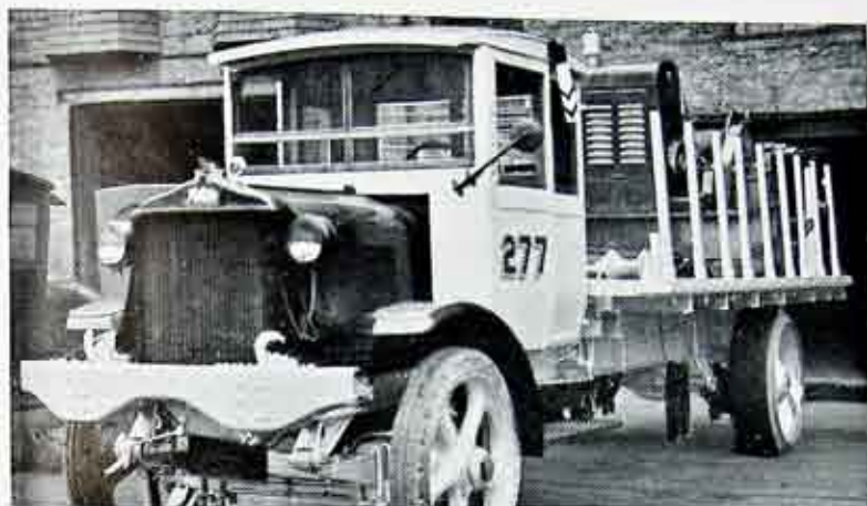
One of the special trucks utilized by Mr. Lamey's men in their varied work, much of which is in connection with the moving or lifting of heavy materials and equipment. This truck body was designed and built by the General Construction Department.
