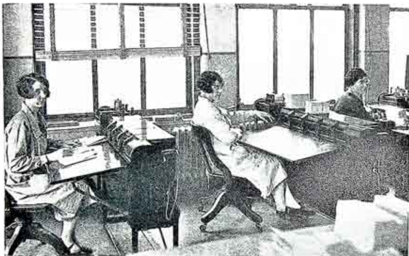
The marvelous electric proving machines receive the punched cards and "work" them, automatically showing the amounts of gas or electricity consumed by customers, in cubic feet or kilowatt hours, respectively; the exact amounts for which customers should be billed and the total number of cards passed through. All totals appear on indicators as the totals are clicked off.
