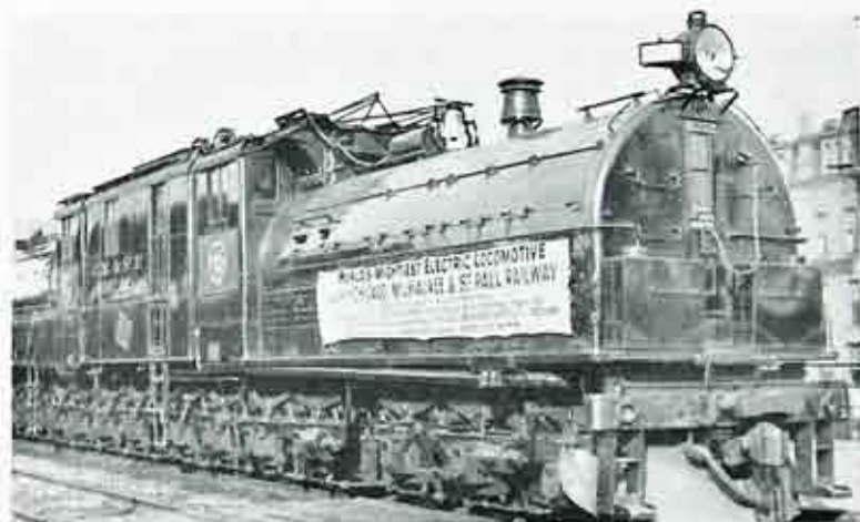
One of Five Electric Locomotives in Use by the Chicago, Milwaukee and St. Paul Railroad. It Weighs 521,000 Pounds and Has an Output of 32,000 Continuous H. P.
