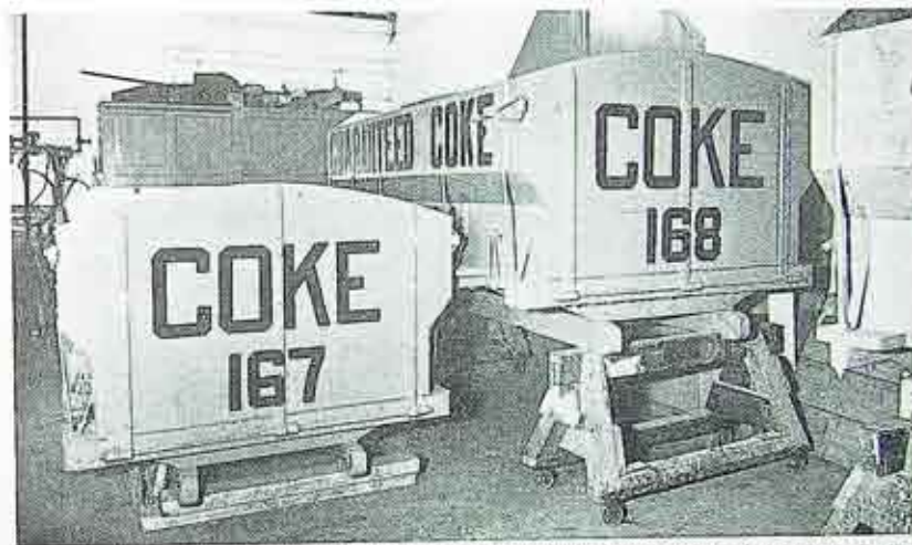
Figure 2. Every Inch of Space is Utilized in the Carpenter Shop. These Coke Truck Bodies Were Constructed and Painted in this Shop, the Portable Skids greatly Facilitating the Process and Insuring the Utilization of Every Square Foot of Floor Space Available.
