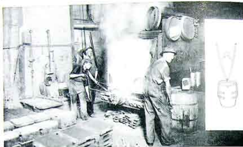
Fig. 2. Pouring brass melted in coal fired brass melting furnaces. Note the clinkers which are adhering to the crucible. Insert shows proper grab tong to be used in lifting the crucible filled with metal from the furnaces.
