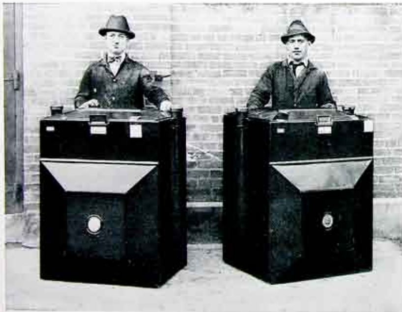
How would you like to have one of these "250 light" (3200 cubic feet per hour) meters installed in your basement? Four of these meters have been installed in a local manufacturing plant
