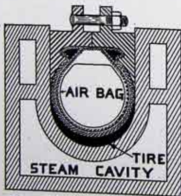
Fig. 2. Cross section of sectional cavity vulcanizer shown in Figure 1
