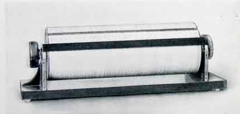
Demand calculating machine used to save time in making out bills for customers on Three Rate Schedule
