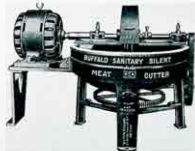
Typical motor-driven cutter used in sausage factory.
