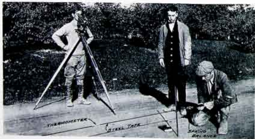
Spring balance shows about 15 pounds pull; man at instrument is reading the measurement on the tape
