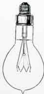
Gas (nitrogen) filled lamp Type C.
