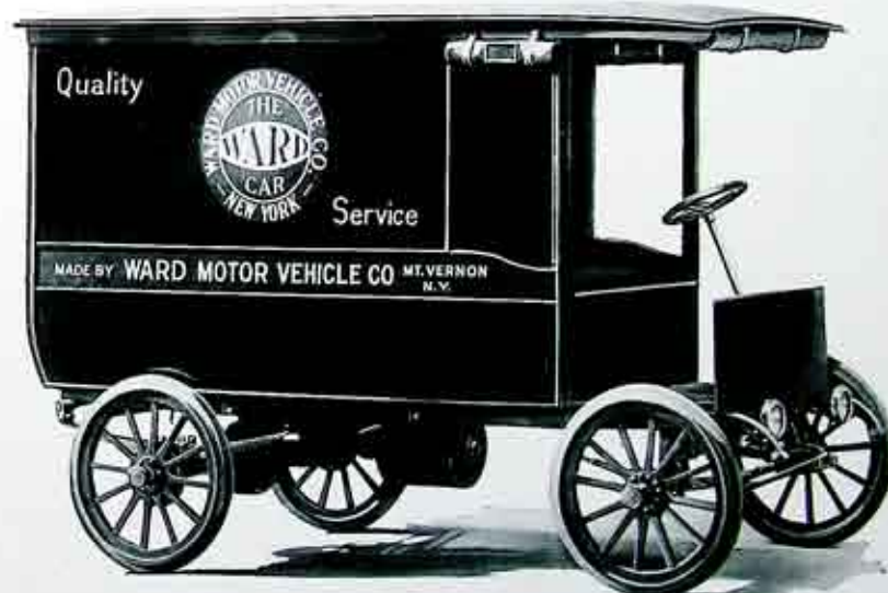
Type of Electric Truck Used by Ward Baking Company
