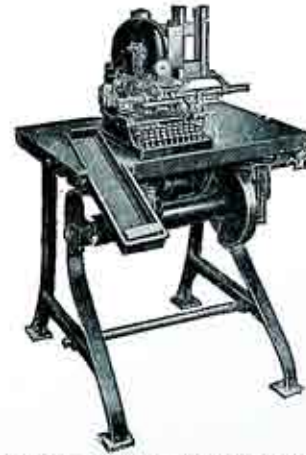
Typograph—Machine used to stencil address plates.
