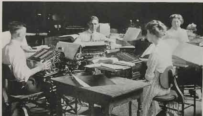
Part of Billing and Posting Group in Consumers' Ledger Department. Burroughs Ledger Posting Machine at left, Billing Machine at Right.
